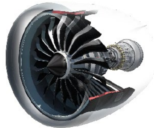
Figure 9: Ultra-High Bypass Ratio engine design (Safran UHBR Clean Sky project)
