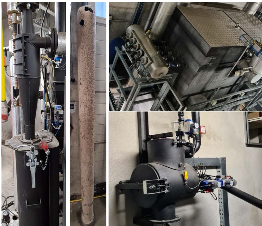
Picture 24: From left to right: cyclone, single cartridge of a cartridge filter, cartridge filter with automatic cleaning device, baghouse filter
