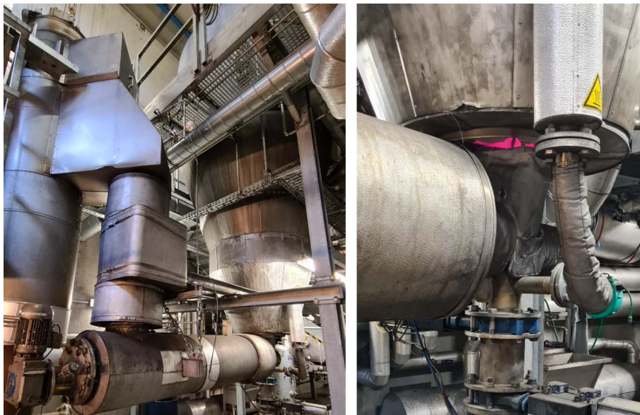
Picture 15: Left updraft pyrolysis with auger screw to move biomass upwards, drop shaft and floating bed reactor; right: bottom of floating bed reactor with oxidation flame and impurities disposal at the base.
