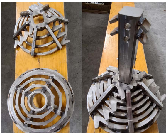
Picture 14: Rotating grate of a fixed bed downstream gasifier: left: taken apart; right: assembled.
