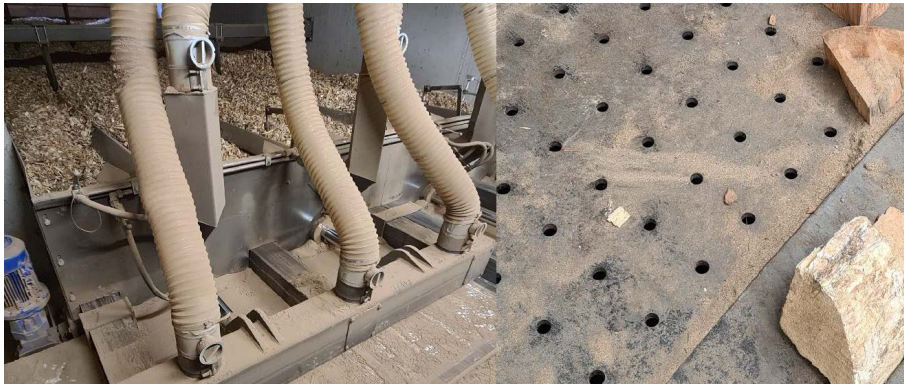
Picture 22: Left: grate dryer with sliding floor and air pipes, right: perforated floor.
