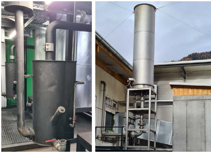
Picture 30: Left: delinking of ambient air to the gasifier via water barrier, right: torch.
