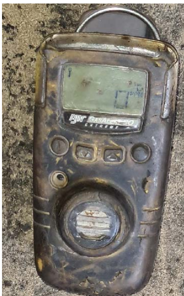
Picture 35: Handheld safety device to detect different types of gases (toxic, explosive).
