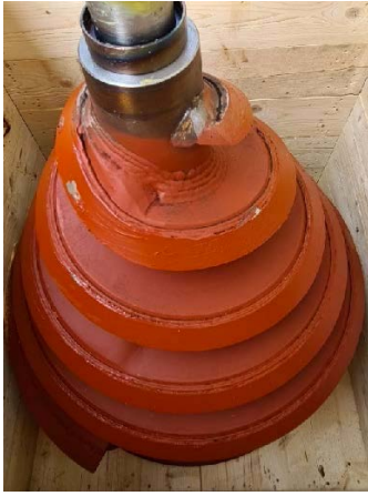
Picture 21: Auger with welded on knife of an auger chipper.
