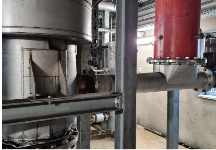
Picture 9: Intake auger screw into an upstream gasifier.
