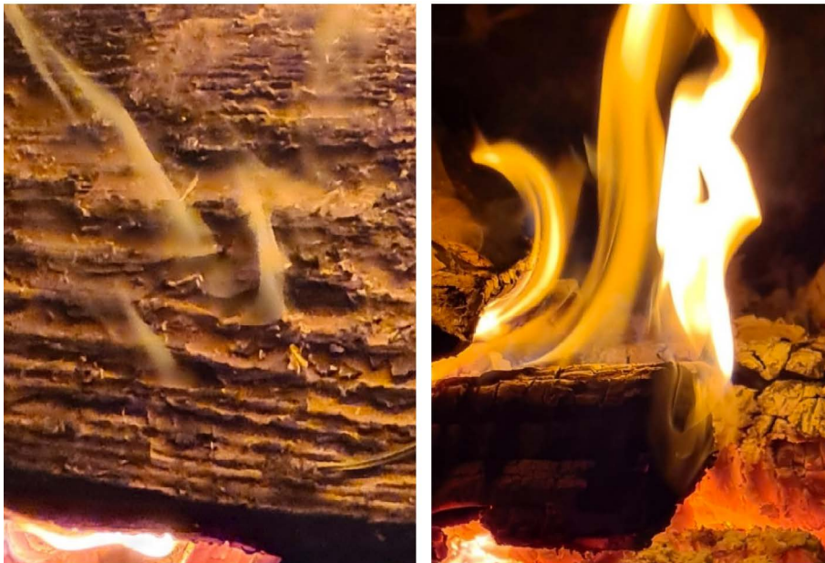
Picture 3: Process steps of biomass combustion: left: gaseous fuel passes out of heated up wooden biomass; right: burning of gaseous fuel.
