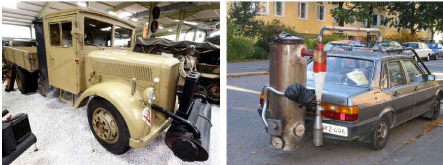
Picture 1: Wood fired gasifier to fuel trucks and cars; left: © AlfvanBeem, right: © Abc10.
