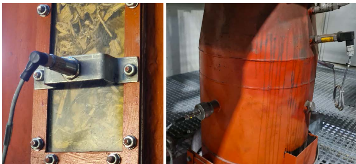
Picture 29: Sensor to check the filling level and to secure the feedstock conveying system.
