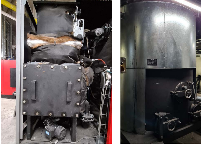
Picture 12: View of fixed bed gasifier; left: 50 kW e , right: 150 kW e . (only bottom part).
