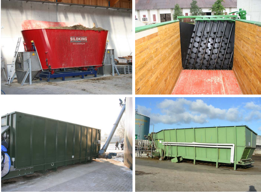
Picture 10: Substrate feeder systems for bulky and dry substrates: top left: with internal mixing screws, top right: feeding system with walking floor, bottom left: push floor, bottom right: scraper floor.
