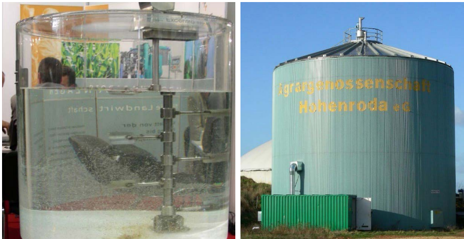
Picture 15: Left: Demonstration object of a continuously stirred digester, right CSTR digester.
