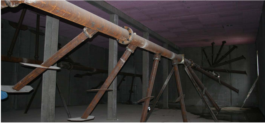
Picture 28: Slow speed agitator in a horizontal digester.
