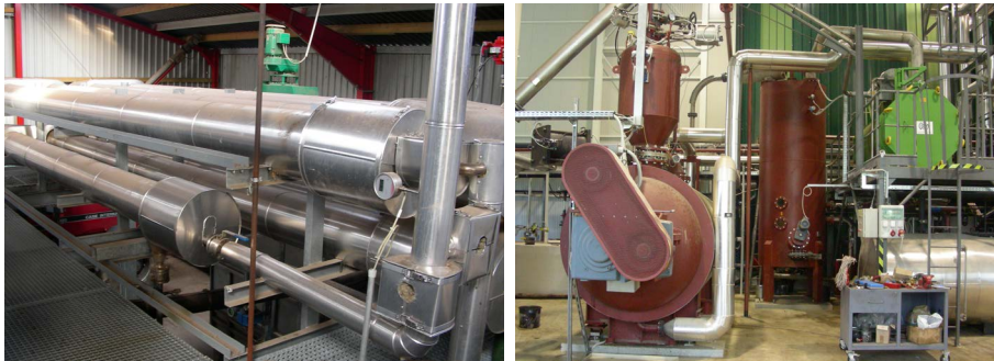
Picture 8: Steam explosion, left: continuously processed, right: batch system.
