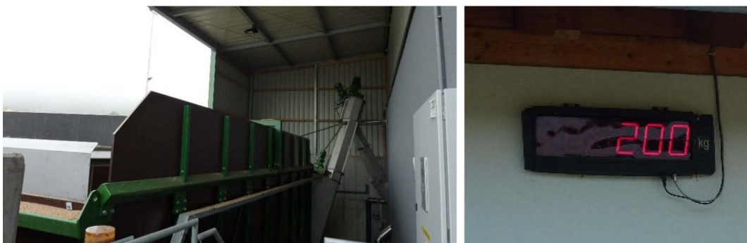
Picture 45: Feeder for bulky substrates with included weighing unit and big display also directly on the device so staff has control when loading the feeder.
