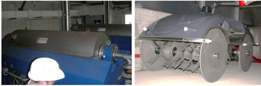
Picture 52: Left: decanter, right: automatically driven digester turner.
