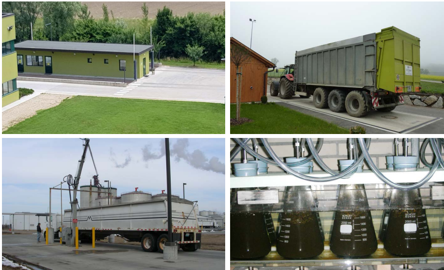
Picture 1: top: office to check delivered feedstock and weighbridge, bottom left: automatic sampling-taking of delivered feedstock, bottom right: batch test determining the methane yield of specific substrates.
