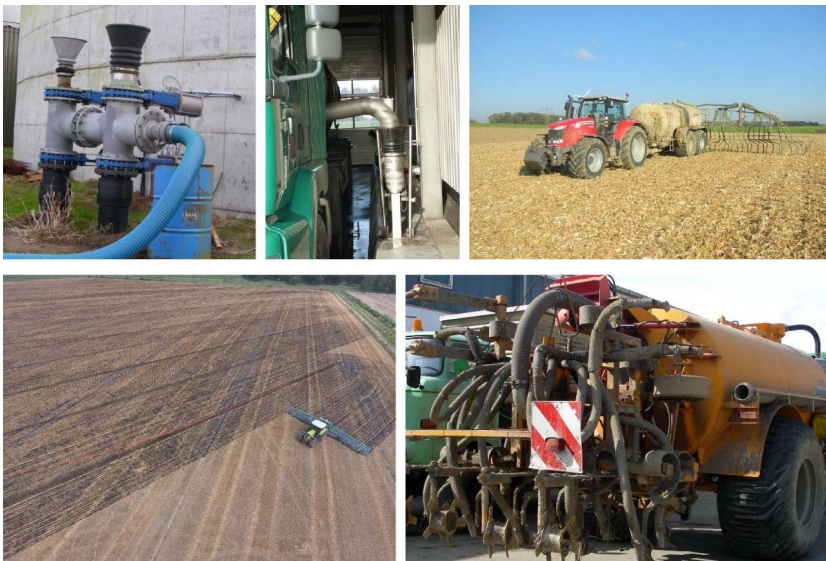
Picture 57: Top: filling station for slurry tanks and slurry tank with trailing hoses; Bottom: slurry spreader without tank and slurry tank with slurry injection.
