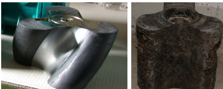
Picture 34: Left: piston of a rotary displacement pump, Right: Damaged piston through impurities like stones.
