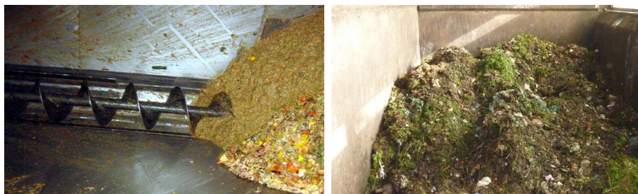
Picture 4: Bunker systems for solid organic waste with two different conveying systems, left: screw conveyor, right: crane.
