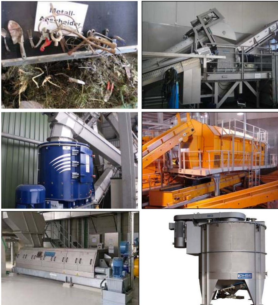
Picture 6: Metal separation is always the first step before further treatment, followed by crushing and further separation like sieving, separation through decanter or pulper. Picture source for sieving and pulper; © Sutco Recycling Technik, Lohse Maschinenbau.
