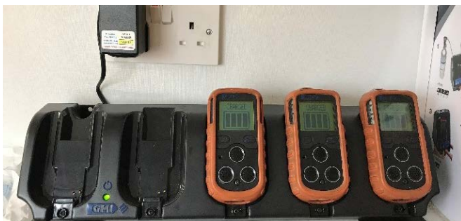
Picture 44: Portable gas detector.
